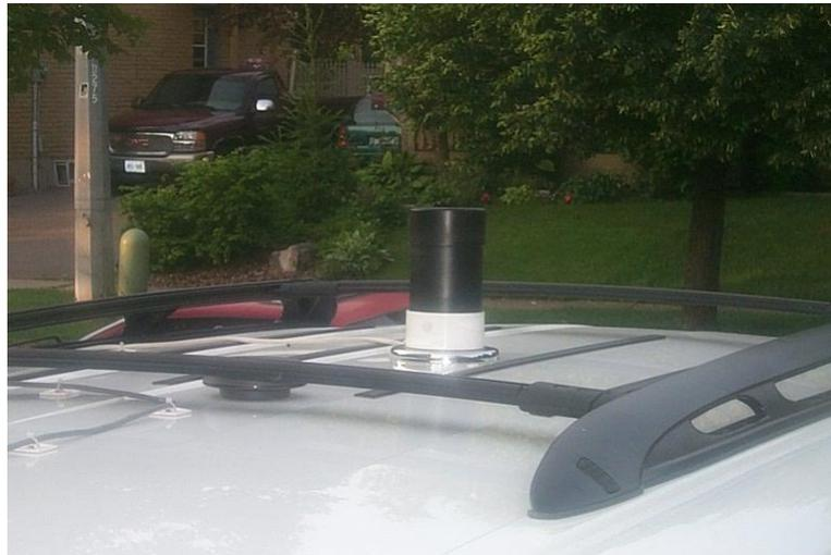
Here the antenna is mounted inside a short piece of PVC sewer pipe purchased from a local hardware store. An end cap covers the top and bottom of the pipe. The antenna is screwed to the side of the pipe with nylon screws. The bottom end cap is screwed to a magnet from a magnetic mount light.
