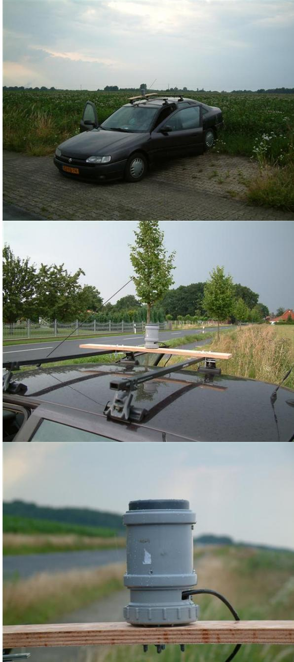
Here the LD-250 antenna is mounted inside a short piece of PVC pipe. Again the components were purchased from a local hardware store.
