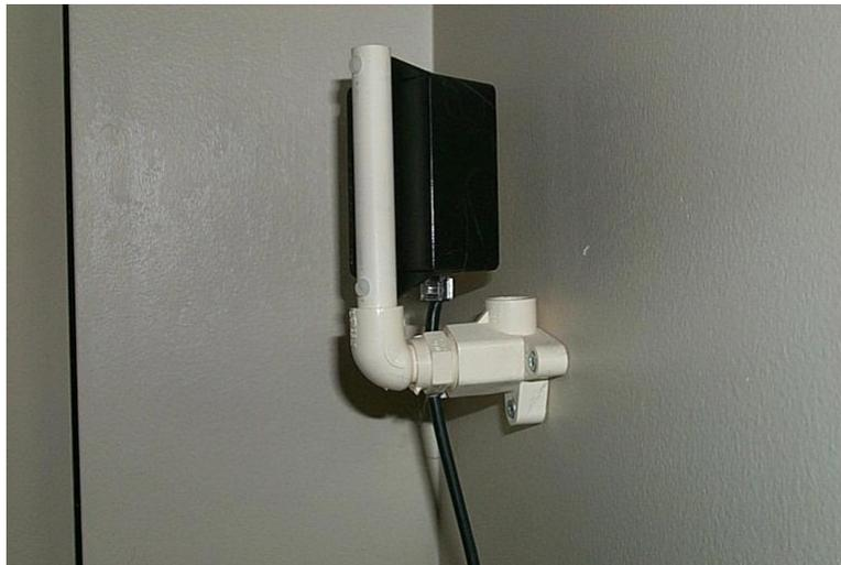
Here the antenna is attached to the drywall in the second floor bedroom of a house. The antenna is mounted on the wall using PVC plumbing hardware purchased at a local hardware store. The antenna is attached to the PVC pipe with nylon screws. The vertical piece of PVC pipe is not cemented so that the antenna can be rotated to fine-tune the direction.
