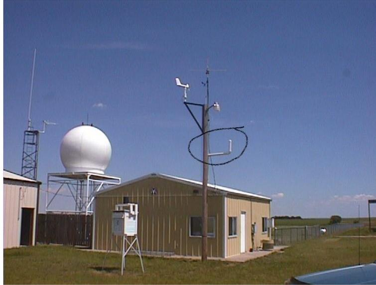
Here the antenna is mounted to the side of a pole using ABS sewer pipe.
