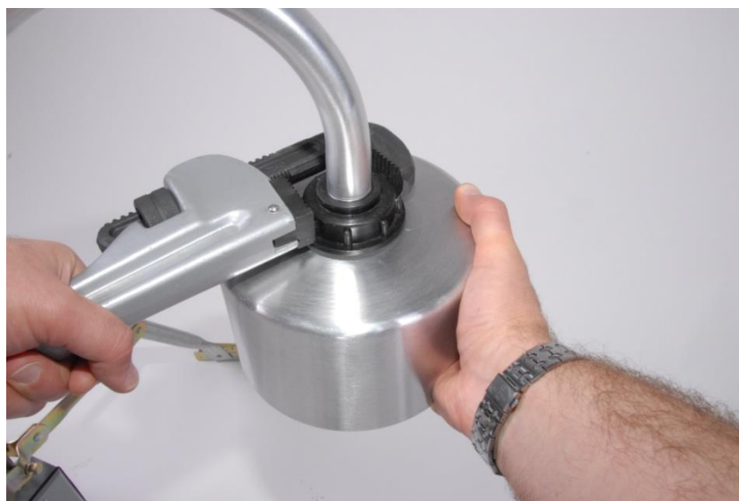
PIPE WRENCH TIGHTENING NUT ONTO RUBBER WASHER (NOTE: LEFT-HANDED COUNTER-CLOCKWISE THREAD ON NUT )
